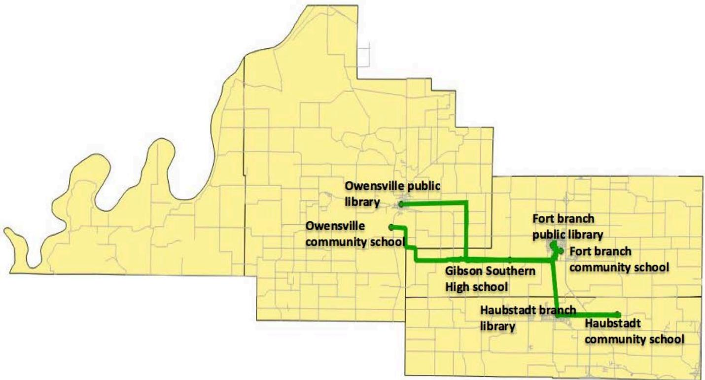
**IMAGE 4 :: THE FINAL REGIONAL BUILDOUT.** A regional 245-mile network serving 5,634 properties would cost an estimated \$11,541,000. With coordinated advance planning between school and municipal officials, the cost of building a 288-strand network throughout the district could be reduced by \$947,000—about eight percent of the total cost.
