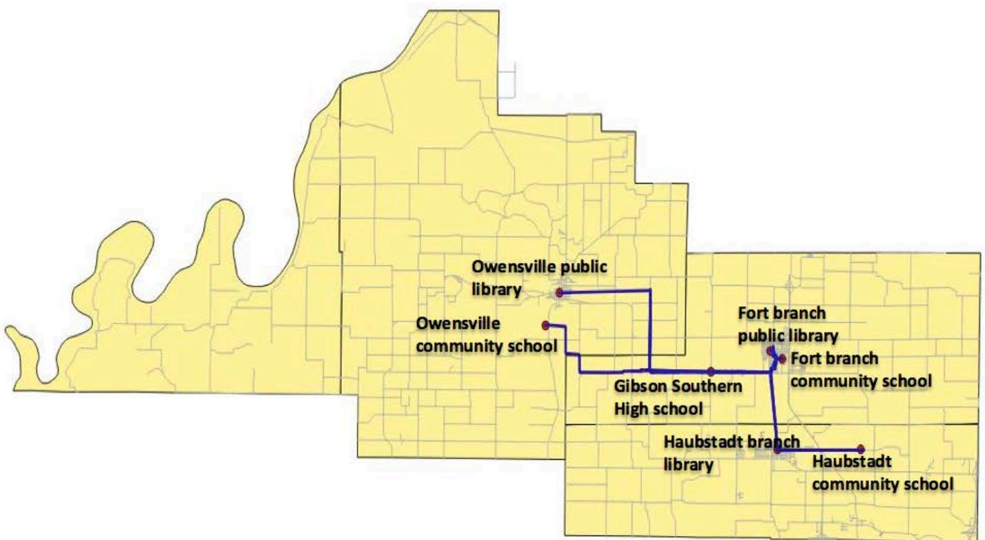
**IMAGE 3 :: COORDINATING AND PLANNING AHEAD.** Increasing the scope of the project from eight strands to 288 strands (fatter line) would cost only an additional \$41,000 in materials, which the municipalities or county could pay to form a portion of a regional public fiber network.
