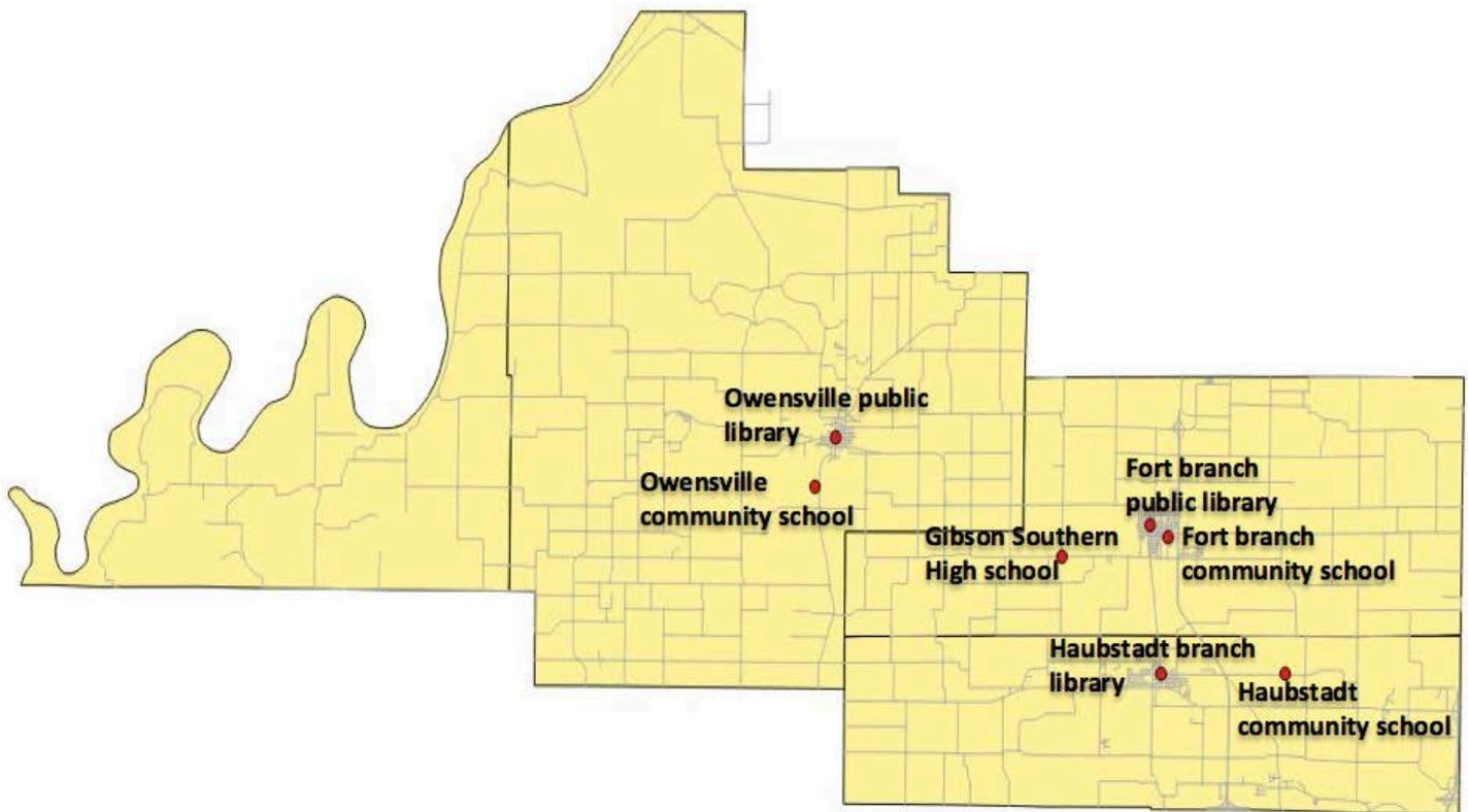
**IMAGE 2 :: A POTENTIAL SCHOOL AND LIBRARY FIBER NETWORK.** Because the rural district has few other options, new E-rate rules might help reimburse the cost of a “self-construction” of 24 miles of fiber to connect these seven buildings. The cost of building eight strands of fiber—enough to serve the schools and libraries—would be \$926,000.
